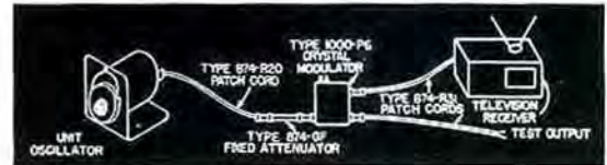
Functional diagram of the unit oscillator with video modulator to form a television signal generator.
