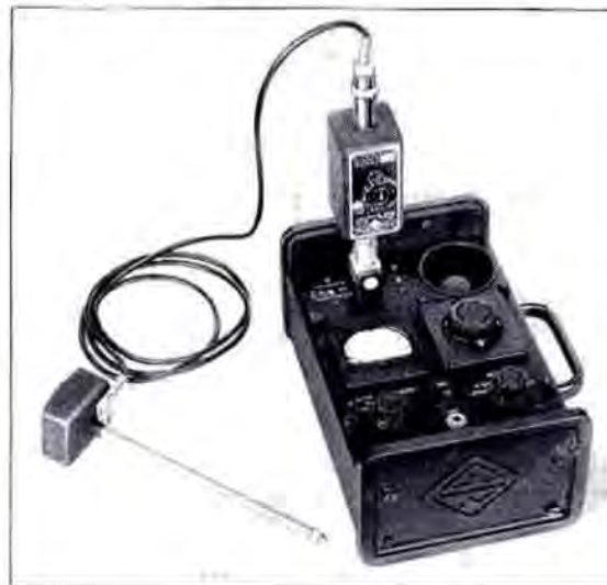
The vibration pickup and control box plug into the sound-level meter in place of the microphone, as shown in the photograph above.
