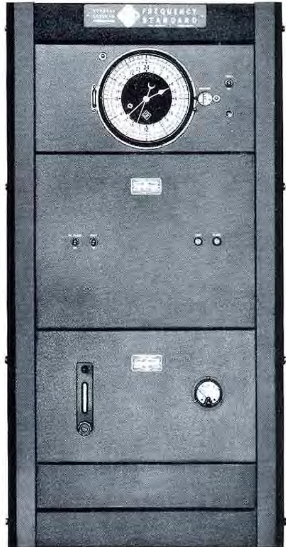
Close-up view of the TYPE 1100-AP Primary Frequency Standard. Lower part of the floor-type relay rack is not shown. The complete rack is similar to that shown in the photograph on page 200. When the standard is to be mounted on a bench or table, a bench-type rack can be supplied, if specified in the order.
