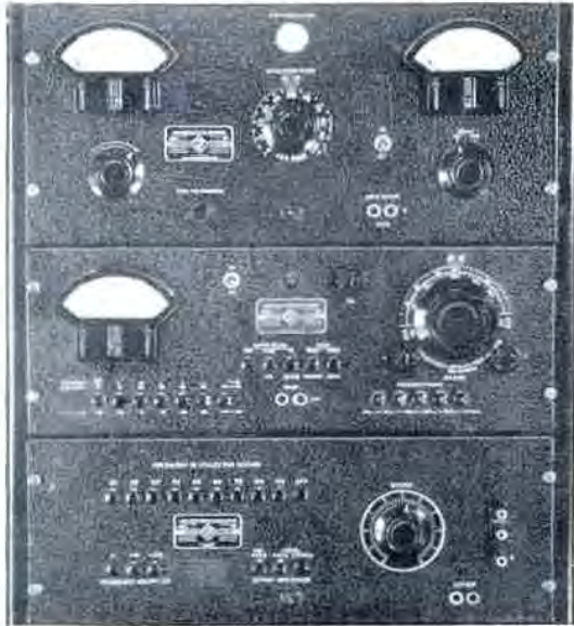
A relay-rack assembly of broadcast test equipment showing, from top to bottom, TYPE 1931-A Amplitude-Modulation Monitor, TYPE 1932-A Distortion and Noise Meter, and TYPE 1301-A Low-Distortion Oscillator.
