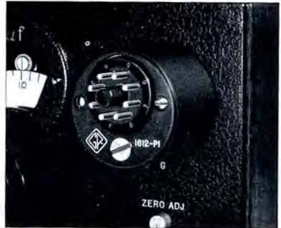
View showing socket adaptor attached to the X terminals of the capacitance meter.
