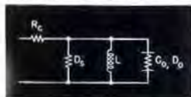
FIGURE A. Equivalent circuit of an air-cored inductor L .
