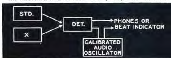
FIGURE 5. Functional diagram showing the operation of the direct-beating method of frequency measurement.
