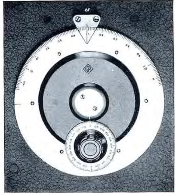
Closeup view of the tuning dial, showing details of the scale.
