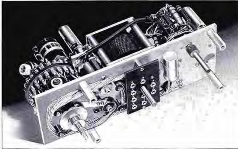
View of the oscillator unit removed from the cabinet. The servicing cable is shown coiled in its storage position. This cable makes possible the operation of the r-f section when it is removed from the cabinet for complete servicing.
